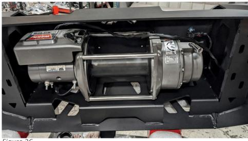
23. If applicable, install your winch using the winch manufacturers provided hardware. (Figure 26)
