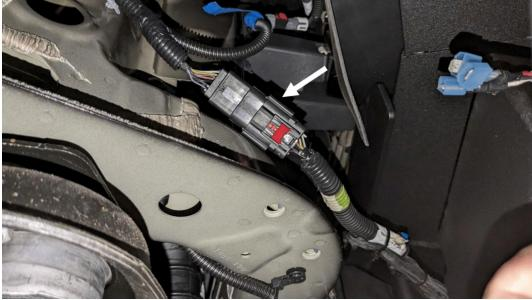
29. Reconnect the parking sensor harness to the vehicle. (Figure 35)
