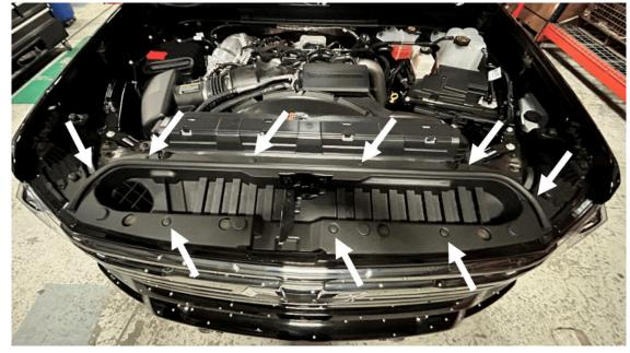
2. Using a panel pry tool, remove the nine (9) push pins retaining the under-hood cowl. Figure 2
