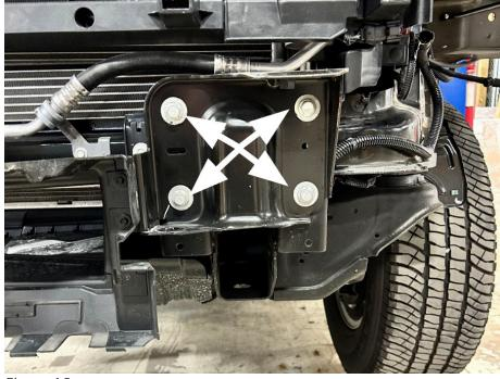
15. Using a 15mm socket wrench, remove the four (4) screws per bumper bracket. Figure 15.
