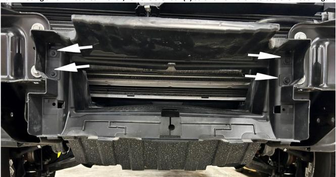
16. Using a 10mm socket wrench, remove the four (4) screws from the intercooler shroud. Figure 17.
