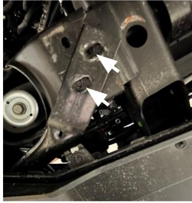
12. Using a 15mm socket wrench, remove the two (2) screws from the bumper gussets. Figure 13.
