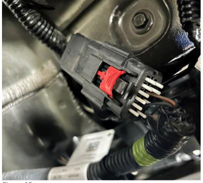
14. Disconnect the bumper electrical wiring harness on the passenger side of the vehicle. Figure 14.
