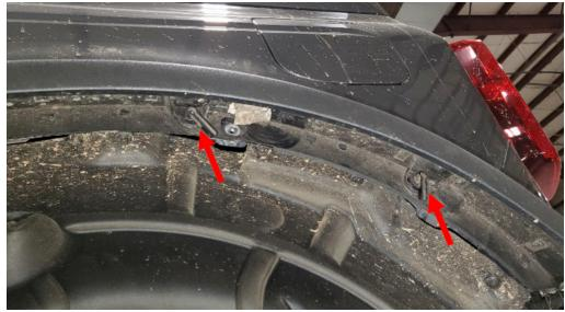
1. Remove factory fender flares by turning plastic levers and pulling off flares. (Figure 1)
