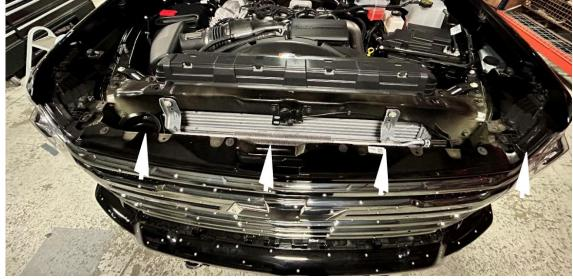
7. Using a 10mm socket wrench, remove the four (4) screws along the top of the grille. Figure 7
