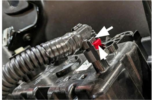
17. Disconnect the bumper wiring harness from each fog light. Figure 19
