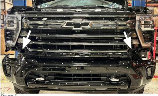
8. Using a 10mm socket wrench, remove the two (2) screws along the bottom of the grille. Figure 8
