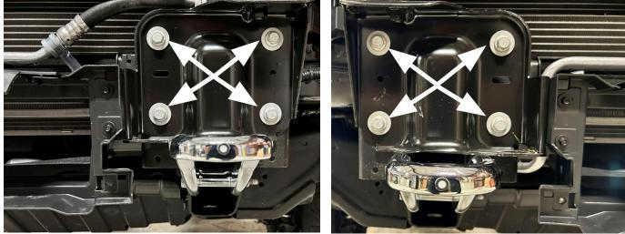
13. Using an 18mm socket wrench, remove the eight (8) bolts per bumper bracket. Figure 14-15
