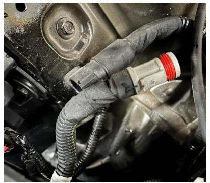
13. If applicable, disconnect the block heater wiring harness on the driver's side of the vehicle. Figure 14.
