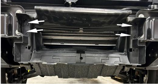
16. Using a 10mm socket wrench, remove the four (4) screws from the intercooler shroud. Figure 17.
