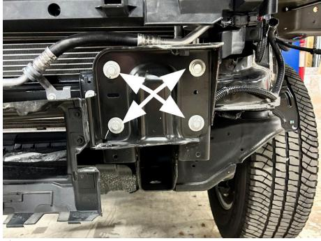
15. Using a 15mm socket wrench, remove the four (4) screws per bumper bracket. Figure 16.
