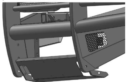
21. After epoxy has fully dried, insert sensors into the housings in the wing and lower guard (23247/23248) in the correct OEM orientation. Route and secure OEM wire harness with zip ties. Figure 23.
