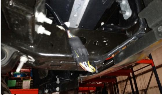
2. Unplug sensors and adaptive cruise control (ACC) from truck wiring harness. Figure 2
