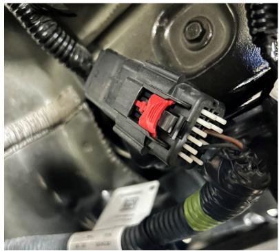
13. Disconnect the bumper electrical wiring harness on the passenger side of the vehicle. Figure 14.
