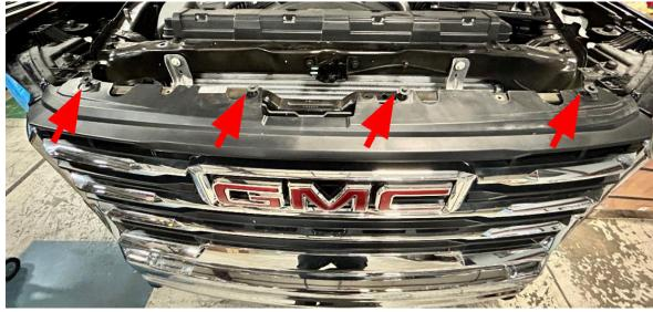
3. Using a 10mm socket wrench, remove the four (4) screws along the top of the grille. Figure 3.
