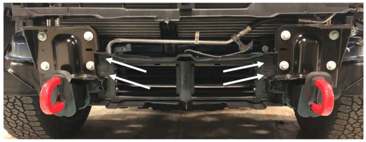
15. Using a 10mm socket wrench, remove the four (4) screws from the intercooler shroud. Figure 16.
