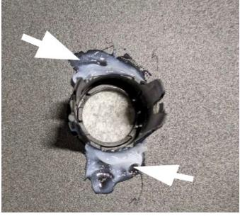
20. Using the provided epoxy, secure all four (4) Oem sensor housings in their appropriate sensor cutout in the bumper (22219). Allow twenty (20) minutes of time for the epoxy to cure. Figure 21
