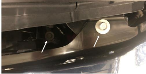
11. Use an 18mm socket wrench to remove four (4) mounting bolts. Figure 12
